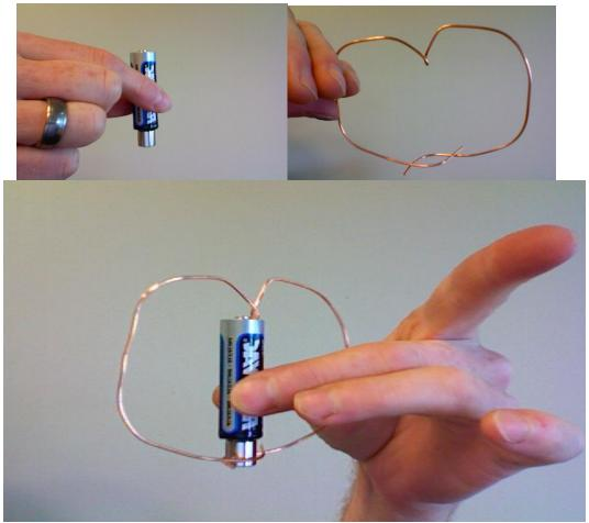
It really helps if the wire has its center of gravity either directly below the point it balances or close to underneath the point it balances on. If the center of gravity is too far off, then the center of gravity will try to shift to directly under the point the
