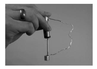
As the charges flow through the wire, the magnet pushes on them when they cross the magnetic field. According to Newton's 3<sup>rd</sup> law (For every action there is an equal and opposite reaction), the charges also push on the magnet. Since the magnet and nail/screw are the only things that can move, they start moving!
