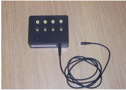
2. DAQ female jack \leftrightarrow PDU (single, side outlet): 6 ft. PDU power cable, male mono connectors
