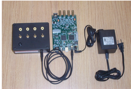
2. DAQ female jack \leftrightarrow PDU (single, side outlet): 6 ft. PDU power cable, male mono connectors
