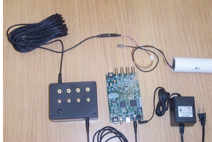
3. PMTs/counters (4) \leftrightarrow PDU (four, side outlets): 50 ft. power extension cable, stereo connectors
