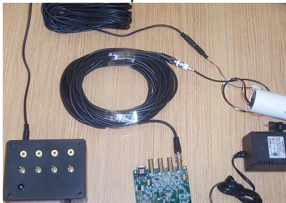
4. PMTs/counters BNC connections (4) \leftrightarrow DAQ BNC connections: 50 ft. BNC signal ext cables
