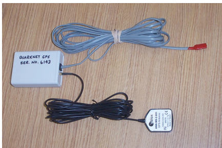
5a. GPS antenna \rightarrow GPS Receiver Assembly: black MCX cable
