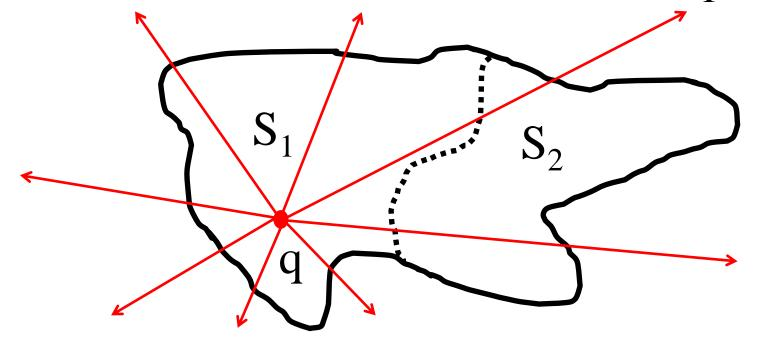
$\Phi_{S} = \Phi_{S_{1}} + \Phi_{S_{2}} \quad \underline{but} \quad \Phi_{S} = \Phi_{S_{1}} = q/\varepsilon_{0}$  $\therefore \Phi_{S_{2}} = 0 \quad (\text{flux into (-) \& out of (+)})$
