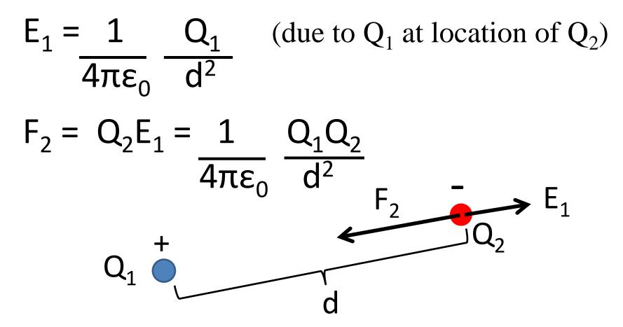
Note: F on a + charge is in direction of E F on a - charge is in the opposite direction
