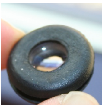
Figure 4: Beam expander lens mounted in rubber grommet
