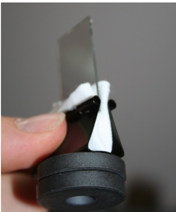
Figure 3: Binder clip with padded Beam Splitter and circular ceramic magnets, the same approach as the non-stage mirror mount
