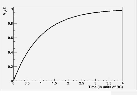
Capacitor in RC circuit charging - voltage vs. time.
