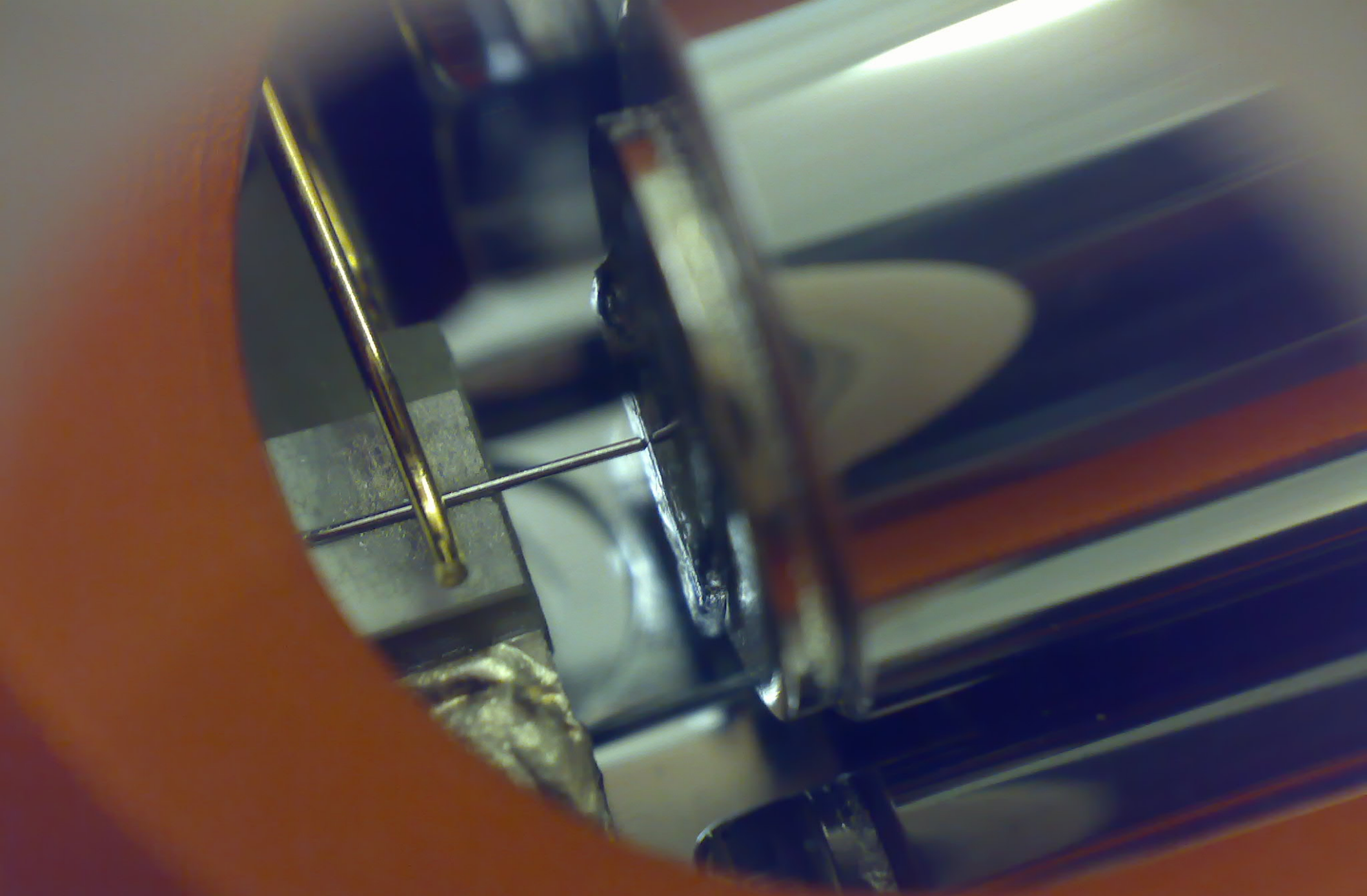
Close-up of a simple scanning-tunneling microscope head using a platinum-iridium stylus
