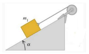
Consider an Atwood machine with mass  $m_1$  on a frictionless ramp with a **MASSIVE** pulley of mass  $m_2$  and moment of inertia of  $I = (2/5)m_2r^2$ . The string is wound around the pulley and does not slip. For coordinates, measure the distance of  $m_1$  along the ramp to be x, and the rotation of the pulley to be  $\theta$ .
