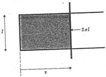
2. The figure illustrates a soap film (shown in gray) supported by a wire frame. Because of surface tension the film exerts a force  $2\sigma\ell$  on the cross wire. This force is in such a direction that it tends to move this wire so as to decrease the area of the film. The quantity  $\sigma$  is called the surface tension of the film, and the factor 2 occurs because the film has two surfaces. The temperature dependence of  $\sigma$  is given by
