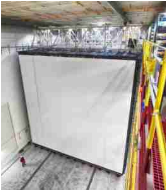
The NOvA detector stands about 50 feet tall and 50 feet wide. (Credit: Fermilab)
