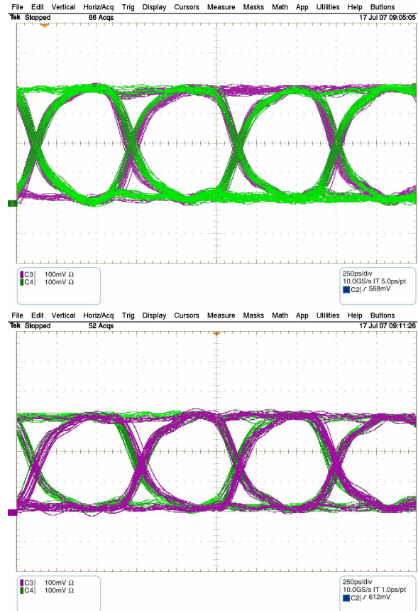
Fig. 4. Serial data waveform (upper: before irradiation; lower: after irradiation with total dose of 100 Mrad(Si)).
