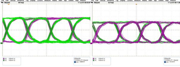
Figure 1: Eye diagram of the GOL serial output before (left) and after (right) the irradiation with 230 MeV protons.
