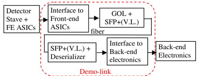
Figure 4: GOL-TLK demo-link block diagram. Shown in the dashed line box is the demo-link, which takes data from the stave and transmit it to the back-end electronics via optical fiber.
