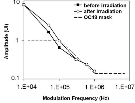
Figure 3: GOL-TLK data link jitter tolerance before and after the irradiation.
