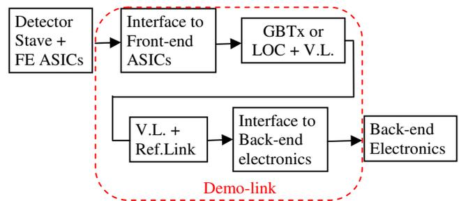
Figure 7: The GBTx or LOC demo-link block diagram. In this design, common projects such as the Versatile Link and the Reference Link are incorporated to minimize the R&D efforts.
