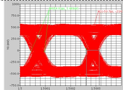
**Figure 6b.** The simulated eye diagram of LOCs1.
