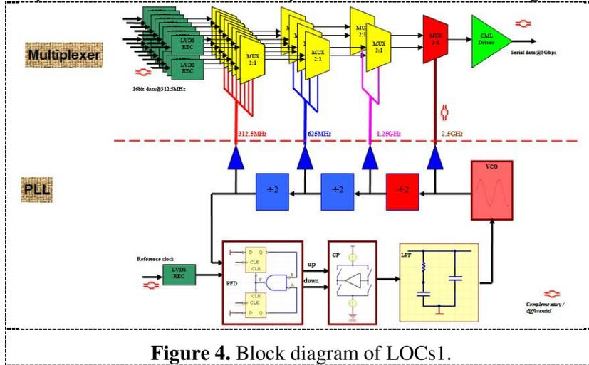
**Figure 4.** Block diagram of LOCs1.
