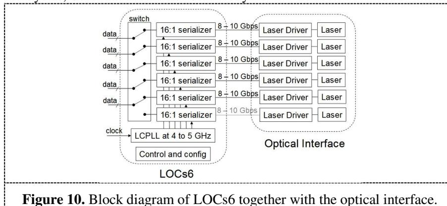
**Figure 10.** Block diagram of LOCs6 together with the optical interface.
