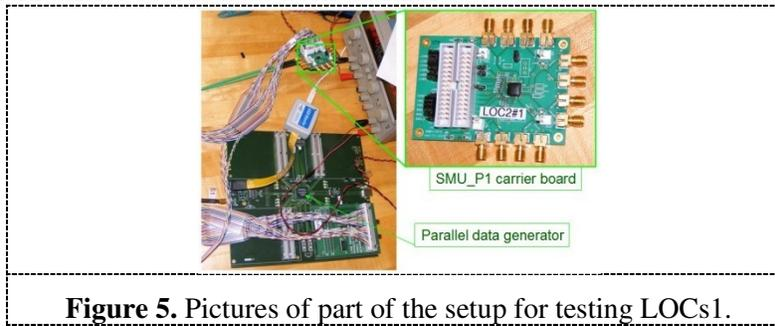
**Figure 5.** Pictures of part of the setup for testing LOCs1.
