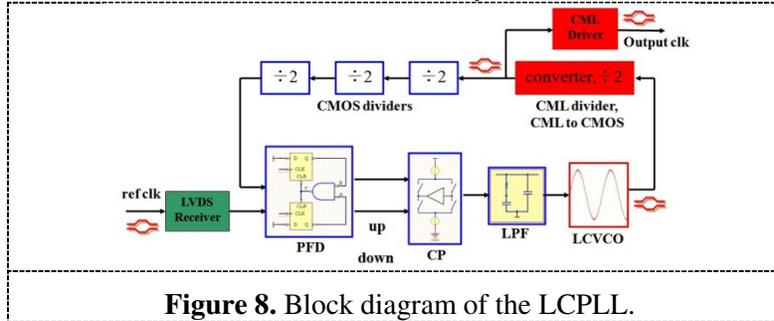
**Figure 8.** Block diagram of the LCPLL.
