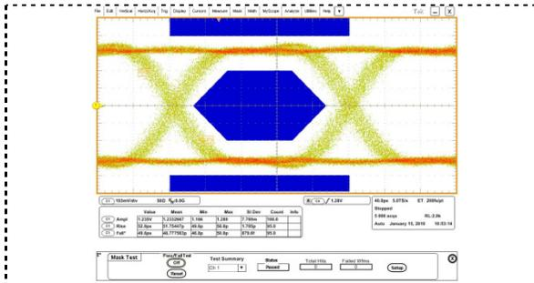
**Figure 6a.** The eye diagram measurement and eye mask test of LOCs1.
