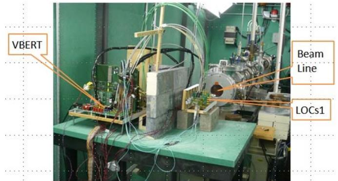
Fig. 7. A picture of the setup of radiation test.
