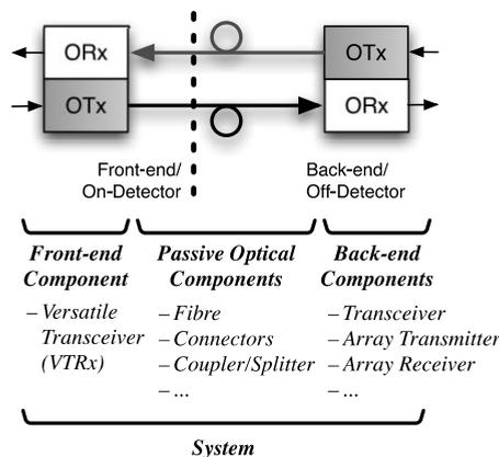
Fig. 1. The Versatile Link architecture.
