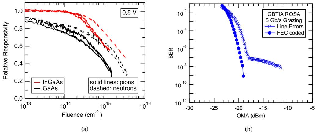
Fig. 4. (a) The effect of 180 MeV pion and 20 MeV neutron irradiation on the responsivity of InGaAs and GaAs photodiodes. (b) The Bit Error Rate induced by a 60 MeV proton beam with a flux of  $2 \times 10^8$  p/cm<sup>2</sup>/s in the GBTIA-based ROSA.
