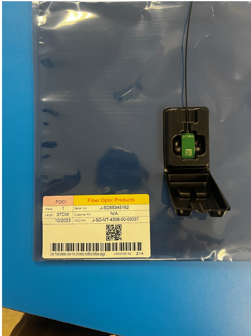
Figure 1.5: The VTRx+ with module id (011849) on its PCB inside opened black plastic case and antistatic bag with pigtail length (37 cm) and pigtail id (J-SD55345162) label.
