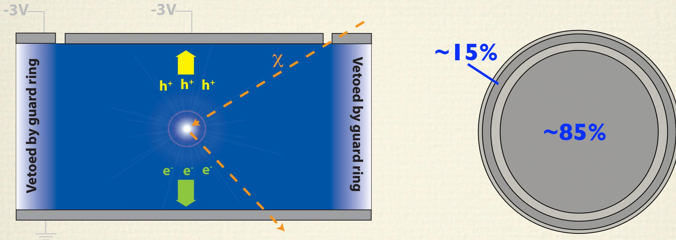
Inner Channel: ionization measurement
