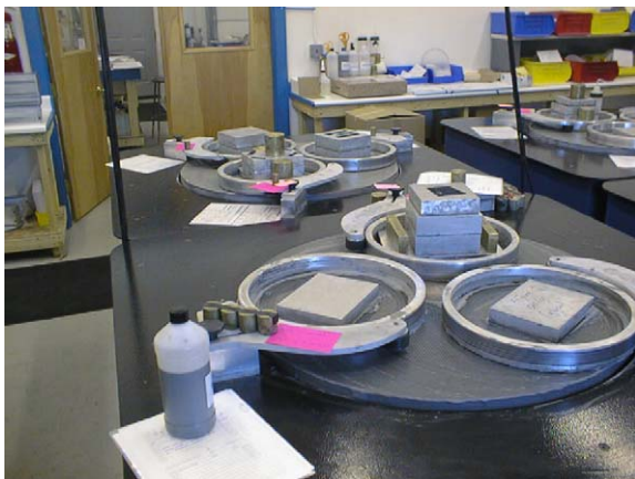
Fig. 7. Photograph of a polishing table, showing the lapping surface and rotating crystal carriers. Weights are placed on the crystals.
