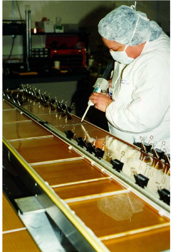
Fig. 20. Construction operations being performed on two multi-wire chambers.
