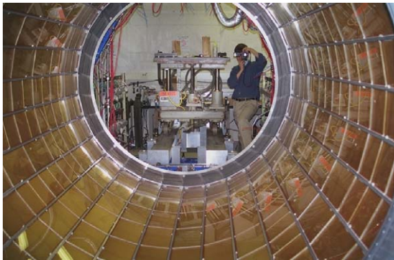
Fig. 26. Photograph of inside of Outer Cylinder with photon detectors installed.
