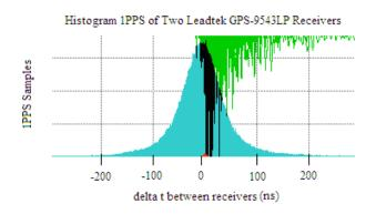
Data analysis is carried out on the time resolution and we find that the GPS module can provide an absolute time measurement with 45 ns resolution. This is good for many physics measurements, like those in cosmic shower array experiments. The spatial data analysis will continue when the new semester starts.
