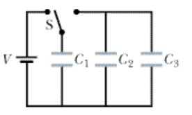
In the figure V = 10 V,  $C_1 = 10$  µF, and  $C_2 = C_3 = 5$  µF.  $R = 10 \Omega$ . Switch S is first thrown to the left side until capacitor 1 is fully charged. Then the switch is thrown to the right. When equilibrium is reached, how much charge is on capacitor 2?
