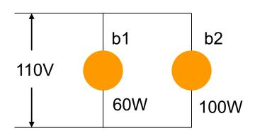
Both bulbs receive the nominal voltage of 110V. They shine as their spec: 60W and 100W. So the 100W bulb is brighter than the 60W.
