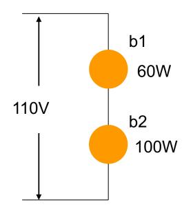
Now the voltage 110V is shared by the two bulbs. The current is the same through them. From  $p = \frac{\Delta V^2}{R}$  One has  $R = \frac{\Delta V_{nominal}^2}{p_{nominal}}$ Then from  $p = I^2 R$ One has  $\frac{p_{b1}}{p_{b2}} = \frac{R_{b1}}{R_{b2}} = \frac{\Delta V_{nominal}^2}{\Delta V_{nominal}^2} = \frac{\Delta V_{nominal}^2}{\Delta V_{nominal}^2}$
