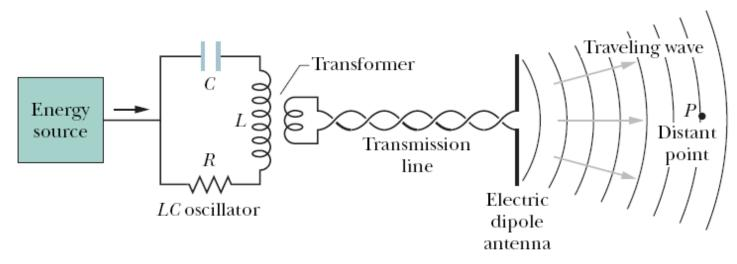
**Fig. 33-3** An arrangement for generating a traveling electromagnetic wave in the shortwave radio region of the spectrum: an LC oscillator produces a sinusoidal current in the antenna, which generates the wave. P is a distant point at which a detector can monitor the wave traveling past it.
