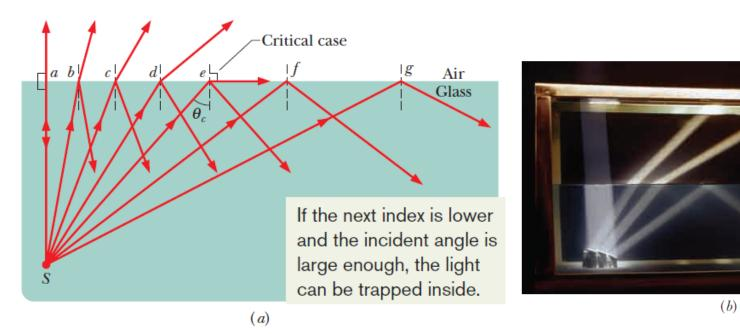
For angles of incidence larger than  $\theta_c$  such as for rays f and g, there is no refracted ray and all the
