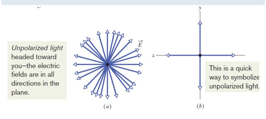
If the intensity of original unpolarized light is  $I_o$ , then the intensity of the emerging light through the polarizer, I, is half of that.
