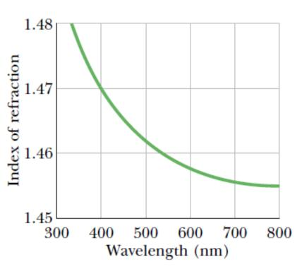
The index of refraction *n* encountered by light in any medium except vacuum depends on the wavelength of the light.
