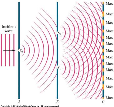
A photograph of the interference pattern of a two slit experiment. The alternating maxima and minima are called interference fringes.
