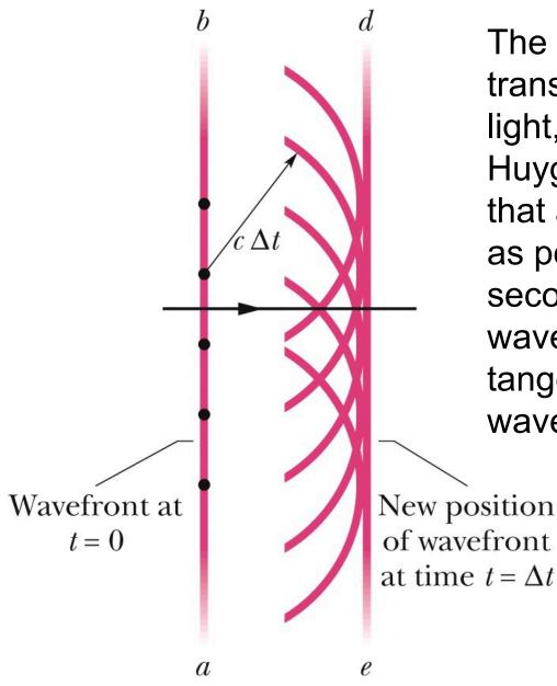
The three-dimensional transmission of waves, including light, may often be predicted by Huygens' principle, which states that all points on a wavefront serve as point sources of spherical secondary wavelets. The new wavefront will be that of the surface tangent to these secondary wavelets.
