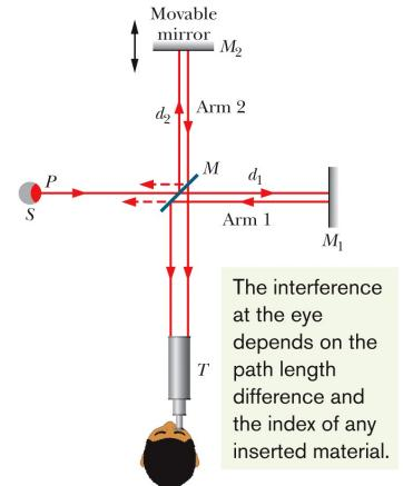
Michelson's interferometer, showing the path of light originating at point *P* of an extended source *S*. Mirror *M* splits the light into two beams, which reflect from mirrors  $M_1$  and  $M_2$  back to *M* and then to telescope *T*. In the telescope an observer sees a pattern of interference fringes.
