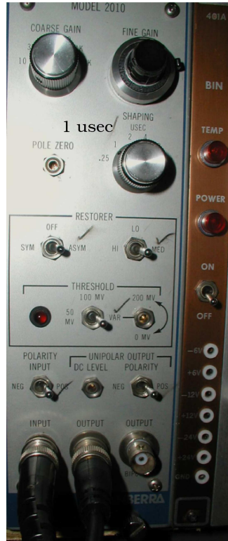
Figure 9: Spectroscopy Amplifier with default settings used for the Compton scattering experiment. Source: Author
