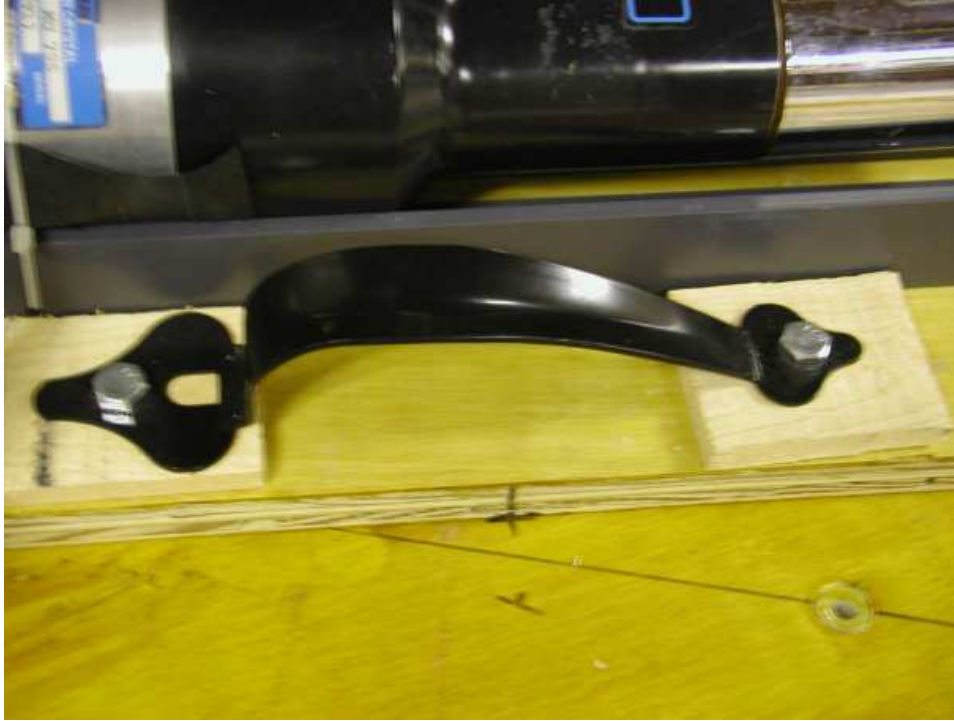
Figure 15: Alignment of the detector housing. In order for the pegs to fit in the placement holes, the hatch marks on both sides of the detector cradle and the platter must line up. Source: Author
