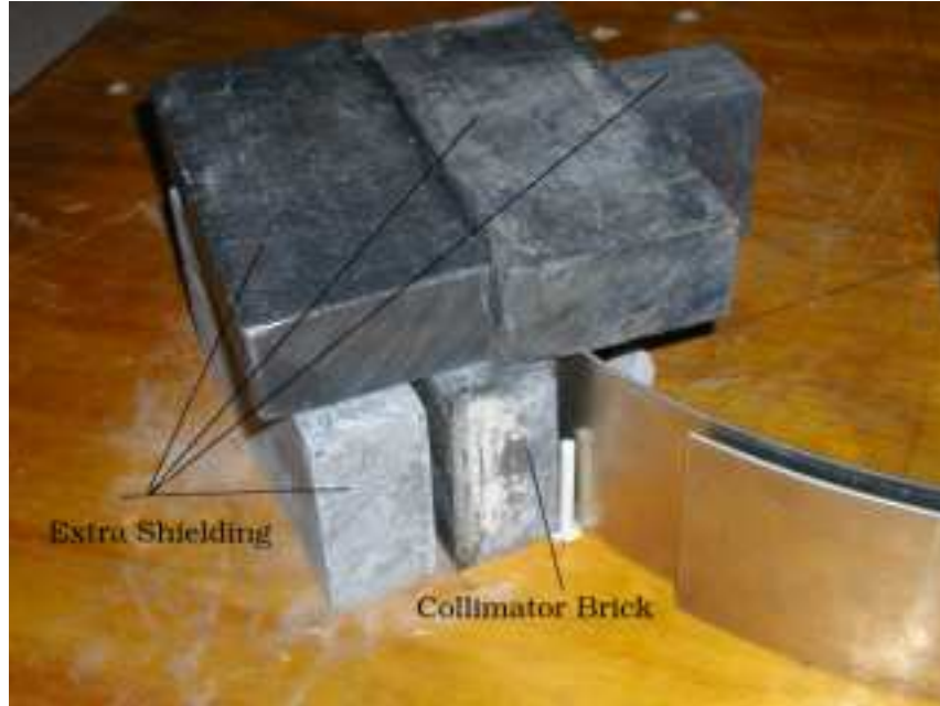
Figure 12: Shielding configuration. The source is held by the collimator brick in the middle of the lead bricks. Source: Author
