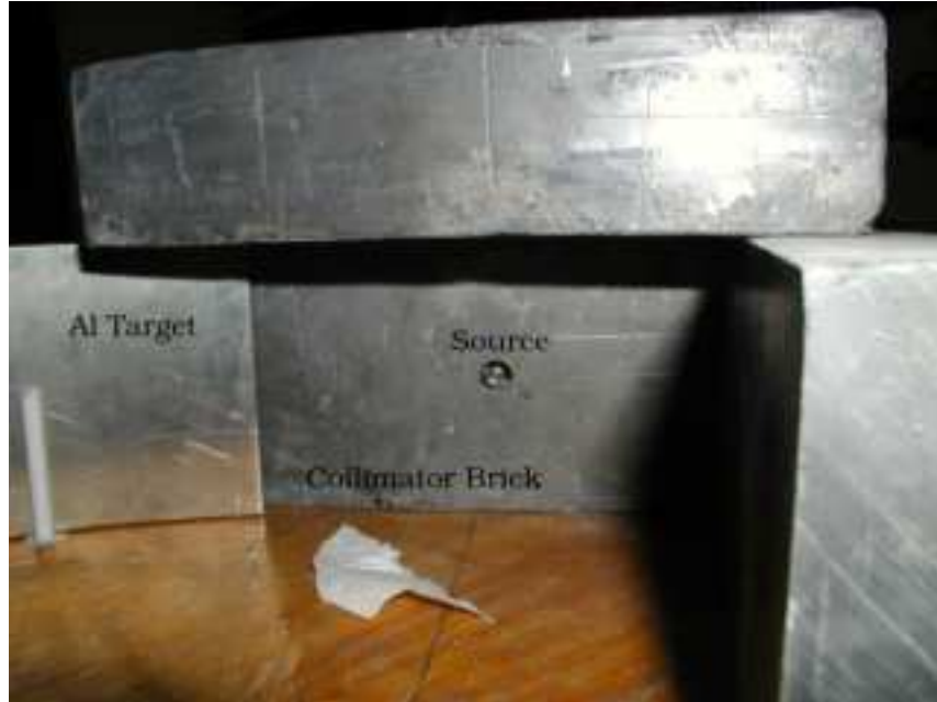
Figure 13: View of source from opposite side of lead shielding. Source: Author
