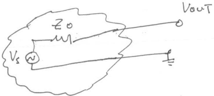
THE CLOUD HIDES THE REAL CIRCUIT WHICH YOU MODEL AS JUST SOME VOLTAGE SOURCE IN SERIES w/ THE OUTPUT IMPEDANCE.
