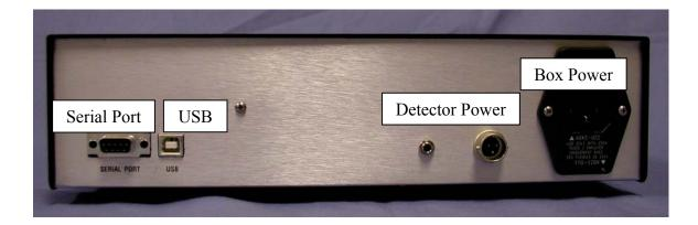
Figure 6. Rear of electronics box. The communications ports are on the left. Use only one.
