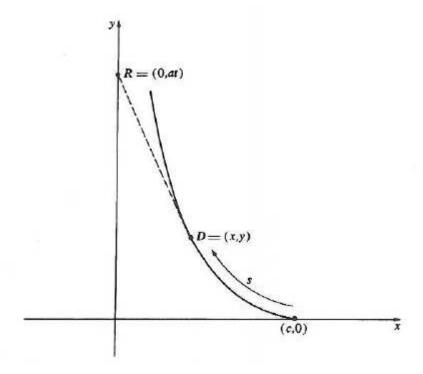
After some time t, the car is at position R = (0, at) and the dog is at position D = (x, y). See the figure. Since the line DR is tangent to the dog's path, we have
