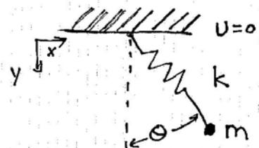
$U=0$  $b = \text{UNSTRETCHED SPRING LENGTH}$  $l = \text{SPRING LENGTH}$
