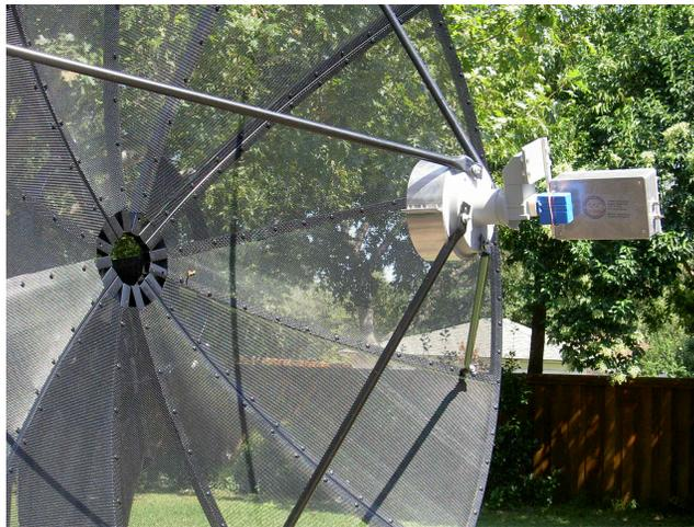
Figure 4: The receiver and feedhorn
