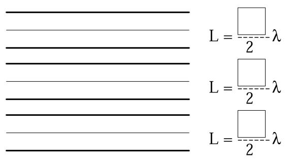
You should observe a pattern. We will now calculate the frequency. If  $L = \frac{N}{2}\lambda$  where  $N = 1, 2, 3, \ldots$  then  $\frac{1}{\lambda} = \frac{N}{2L}$ . Using  $v = f\lambda$ , we have:
