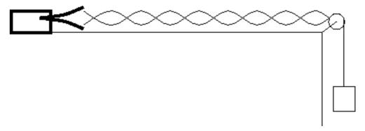
Adding mass to the hanger will change the tension in the string. This will change the wave speed in the string. With the frequency and string length fixed throughout the experiment, we will generate different standing wave modes with different wavelengths. We will measure the wavelengths of the various standing waves and find the relationship between tension and wavelength.
