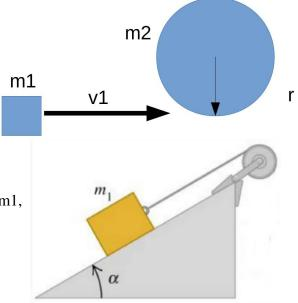
3) Consider the figure at right. The pulley is friction-less, but has mass  $m_2$  and moment of inertia  $I=(1/2)m_2r^2$ . The block has mass m1, and slides on a friction-less surface with angle  $\alpha$ .
