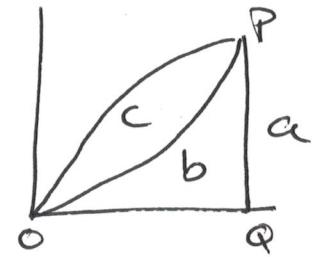
$$\begin{aligned} @ &= \int_0^Q dx + \int_Q^P dy = \int_0^1 dx F_x(x, 0) + \int_0^1 dy F_y(1, y) \\ &= \int_0^1 dx (x^2) + \int_0^1 dy (2y) = \left[ \frac{x^3}{3} \right]_0^1 + \left[ \frac{2y^2}{2} \right]_0^1 = \frac{4}{3} \end{aligned}$$
