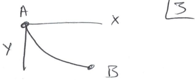
$$\text{time} = \int_A^B dt = \int \frac{ds}{v} = \int \frac{\sqrt{dx^2 + dy^2}}{\sqrt{2gy}} = \int \frac{\sqrt{\frac{dx^2}{dy^2} + 1}}{\sqrt{2gy}} dy$$
