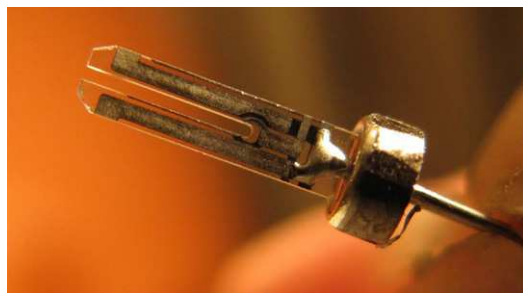
Figure 2: Magnified image of a quartz crystal cut into the shape of a tuning fork used in quartz clocks. From Ref 3.
