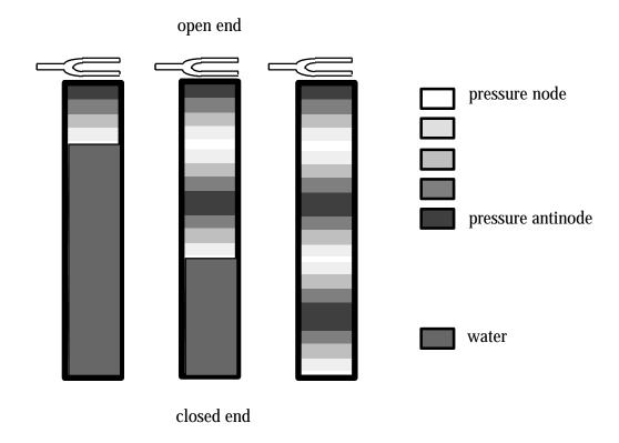
By this method, its length (L) may be "tuned" to resonate with a tuning fork of known frequency. From the above condition for resonance, one can determine the wavelength of the resonances, and if the frequency of the tuning fork is given, one may use the following relationship to calculate the velocity of sound:
