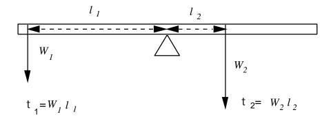
After this, we will place the fulcrum at some point away from the center of the meter stick and repeat the process. Since all of the mass is effectively concentrated at the center of gravity, one must account for the torque resulting from gravity acting on the meter stick. Balancing the meter stick in this manner will make it possible to determine its weight.
