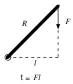
The two cases drawn above have the same torque. The drawing on the right shows how to find the lever arm when the force is not perpendicular to the rod. The case in the diagram is similar to the use of a wrench in tightening a bolt. If the force were in the same direction as the wrench, the bolt would never turn. If the force was perpendicular to the wrench, then l would equal R and the torque would be greater than in the diagram.
