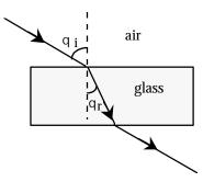
The **law of refraction** or **Snell's law** describes the amount of refraction which will take place. This law states that the index of refraction of the incident medium multiplied by the sine of the incident angle is equal to the index of refraction of the refracting medium multiplied by the sine of the refracted angle.
