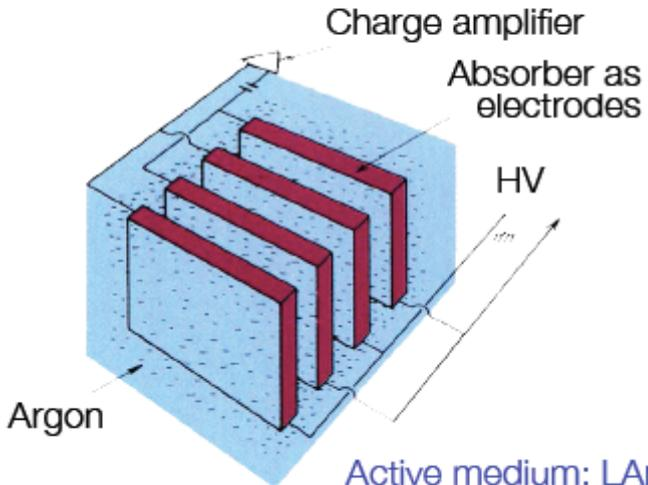
Active medium: LAr; absorber embedded in liquid serve as electrodes
