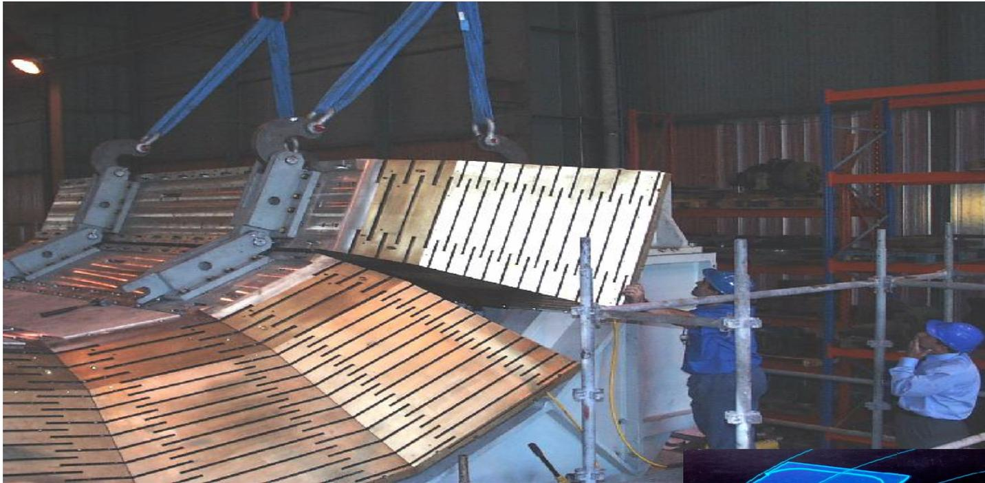
Scintillators fill slots and are read out via fibres by HPDs
