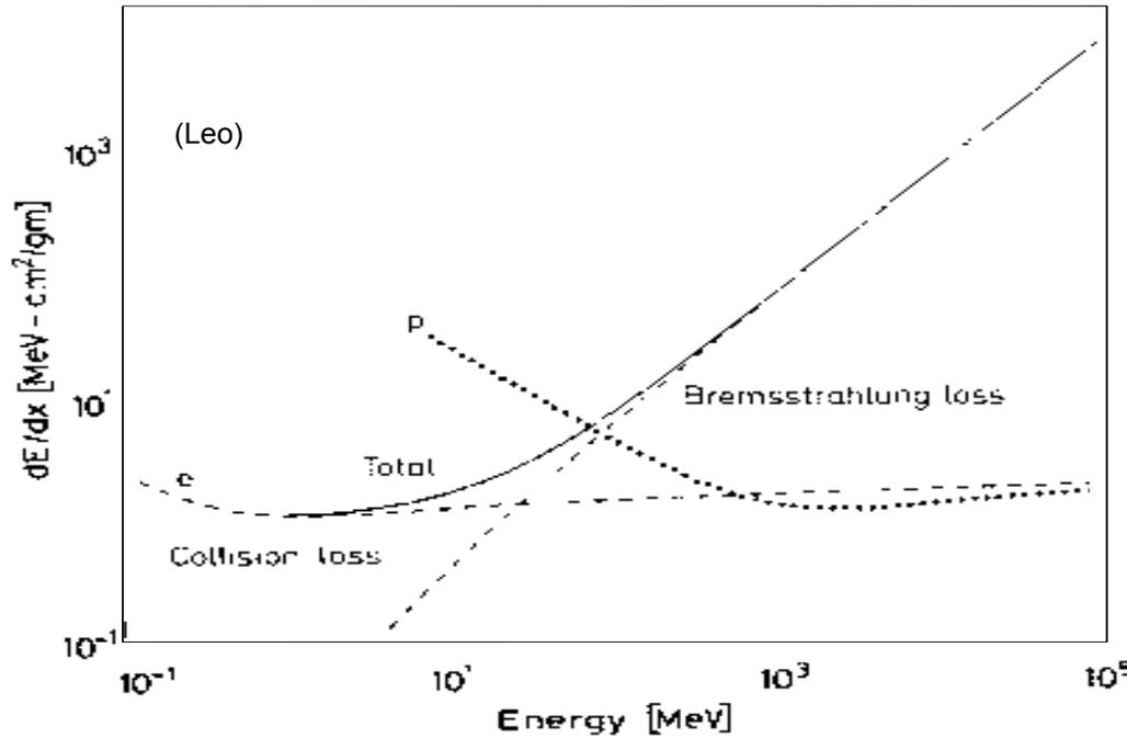
energy loss (radiative + ionization) of electrons and protons in copper
