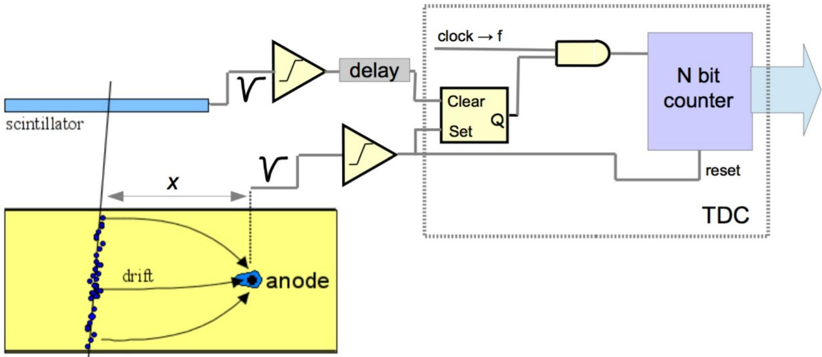
Single Hit TDC: If a noise pulse hits before the signal - the measurement is lost
