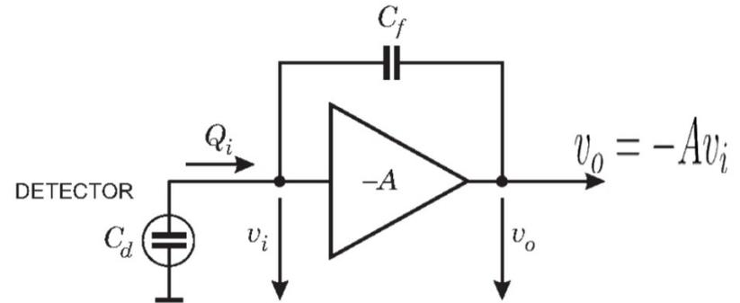
$$A_Q = \frac{v_o}{Q_i} = \frac{Av_i}{C_f(A+1)v_i} = \frac{A}{A+1} \frac{1}{C_f} \approx \frac{1}{C_f} \quad (A \gg 1)$$
