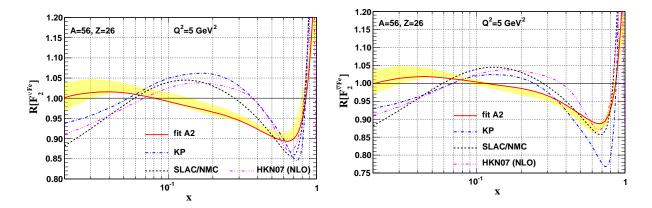
Figure 3: Nuclear correction factor R for the structure function  $F_2$  in a) neutrino and b) anti-neutrino scattering from Fe. The solid curve shows the result of our analysis of NuTeV data; the uncertainty from the fit is represented by the shaded (yellow) band. For comparison we show the correction factor from the Kulagin-Petti model (dasheddot line),  $^4$  HKN07 (dashed-dotted line),  $^5$  and the SLAC/NMC parametrization (dashed line).  $^2$
