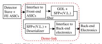
Figure 4: GOL-TLK demo-link block diagram. Shown in the dashed line box is the demo-link, which takes data from the stave and transmit it to the back-end electronics via optical fiber.
