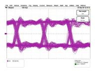
Figure 6: Optical eye diagram of measured from the GOL-TLK demo-link.
