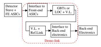
Figure 7: The GBTx or LOC demo-link block diagram. In this design, common projects such as the Versatile Link and the Reference Link are incorporated to minimize the R&D efforts.
