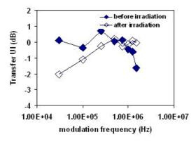
Figure 2: GOL jitter transfer function before and after the irradiation.
