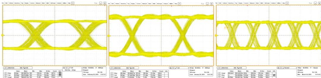
Fig. 4. (a) the eye diagram at room temperature and nominal voltage; (b) the eye diagram at 77 K and nominal voltage; (c) the eye diagram at 77 K and 1.8 V
