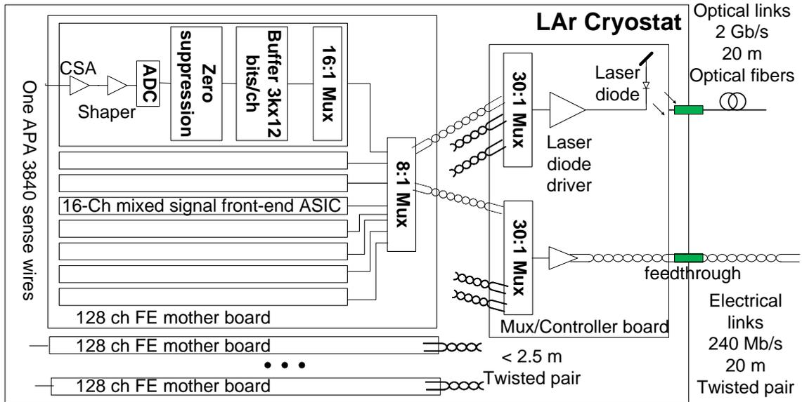
Fig. 1. The block diagram of the front-end electronics with optical data links
