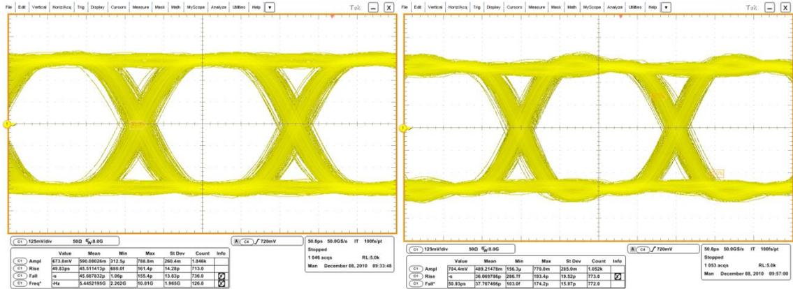
Fig. 5. (a) eye diagram at room temperature; (b) eye diagram at 77 K;
