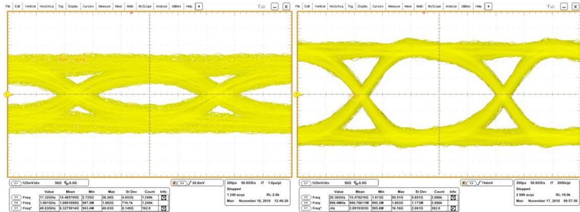
Fig. 3. (a) eye diagram at 1 Gbps and room temperature; (b) eye diagram at 1 Gbps and 77 K
