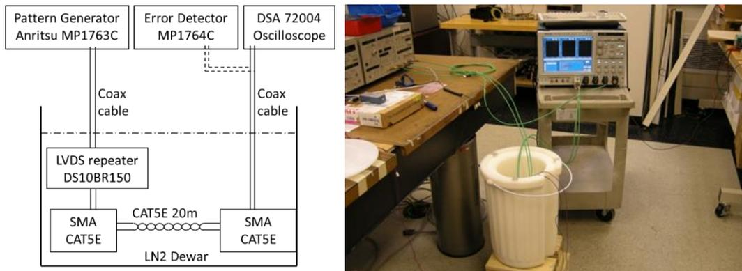
Fig. 2. (a) the block diagram of the test setup; (b) a picture of the test setup
