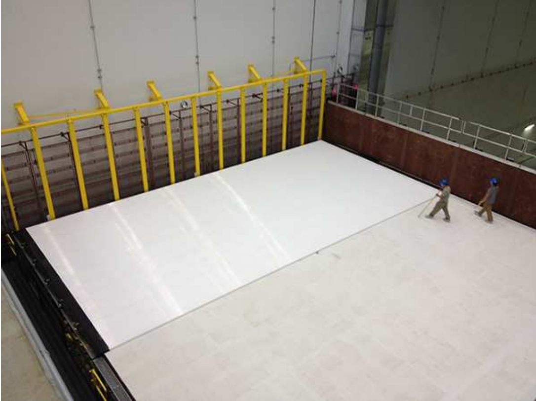
FIG. 2: View looking down on several modules placed on the block pivoter table. The laser scanner is above the table, out of view.
