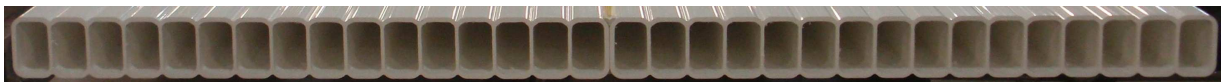
FIG. 1: A cross-sectional view of a 32-channel module. The top and bottom surfaces of the extrusions are flat in a region directly above and below a cell center. The eventual neutrino beam direction is in the plane of the paper and parallel to the longer pair of cell walls.
