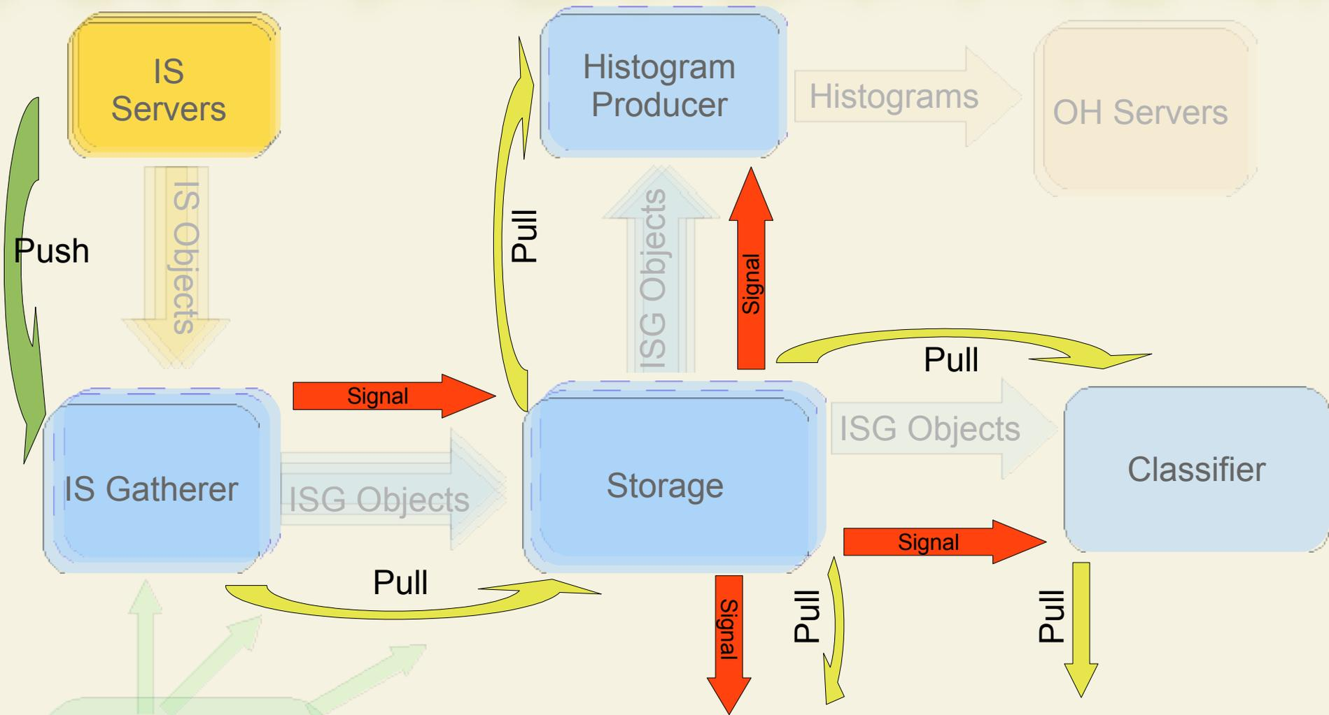
Push-Pull approach in combination with signaling mechanism permits parallel design thus allowing a high level of concurrent processing.
