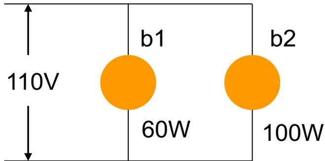
Both bulbs receive the nominal voltage of 110V. They shine as their spec: 60W and 100W. So the 100W bulb is brighter than the 60W.
