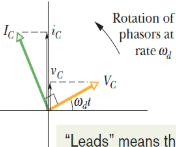
“Leads” means that the current peaks at an *earlier* time than the potential difference.
