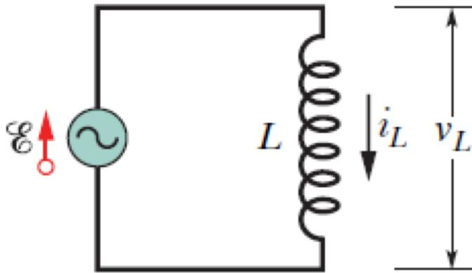
The value of  $X_L$ , **the inductive resistance**, depends on the driving angular frequency  $\omega_d$ . The unit of the inductive time constant  $\tau_L$  indicates that the SI unit of  $X_L$  is the *ohm*.
