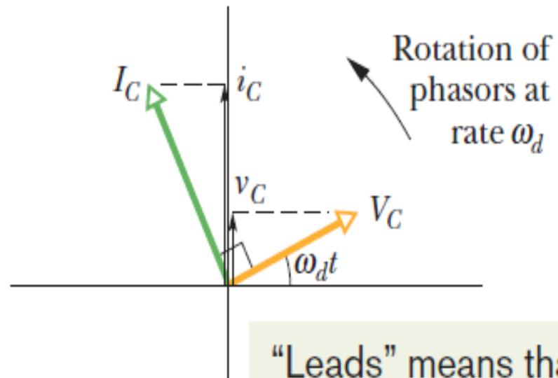
“Leads” means that the current peaks at an *earlier* time than the potential difference.
