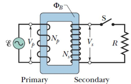
**Fig. 31-18** An ideal transformer (two coils wound on an iron core) in a basic transformer circuit. An ac generator produces current in the coil at the left (the *primary*). The coil at the right (the *secondary*) is connected to the resistive load  $R$  when switch  $S$  is closed.
