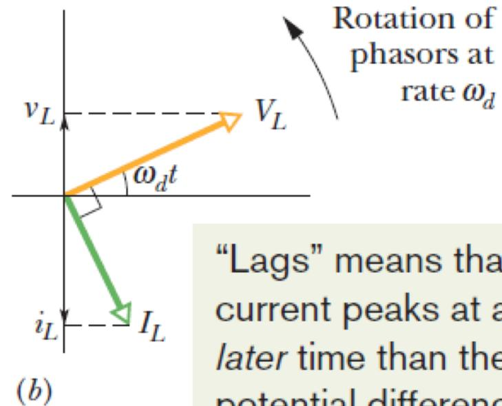
“Lags” means that the current peaks at a *later* time than the potential difference.
