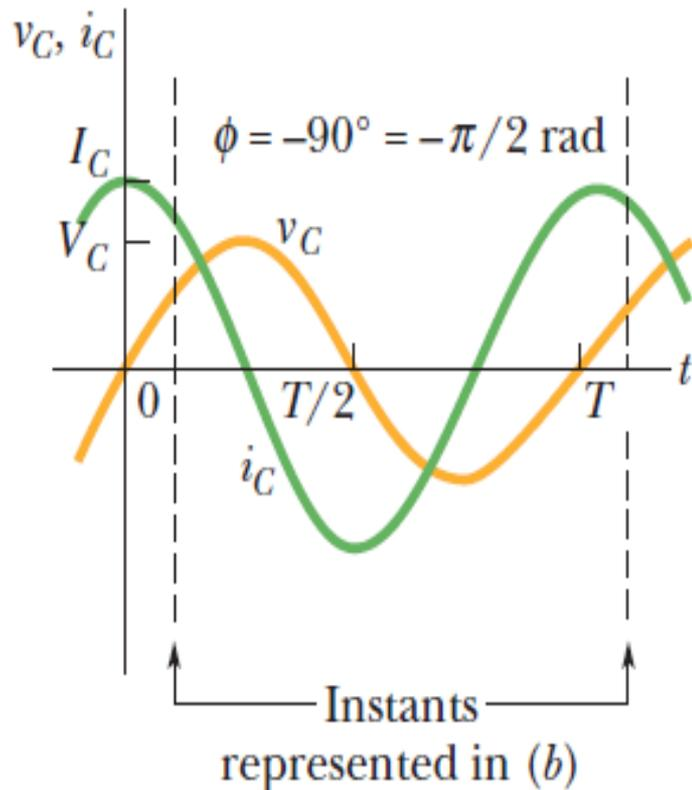
The current in the capacitor leads the voltage by  $90^\circ$
