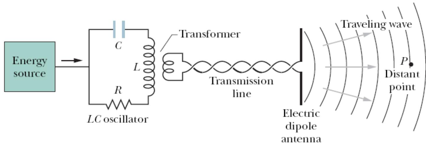
**Fig. 33-3** An arrangement for generating a traveling electromagnetic wave in the shortwave radio region of the spectrum: an  $LC$  oscillator produces a sinusoidal current in the antenna, which generates the wave.  $P$  is a distant point at which a detector can monitor the wave traveling past it.
