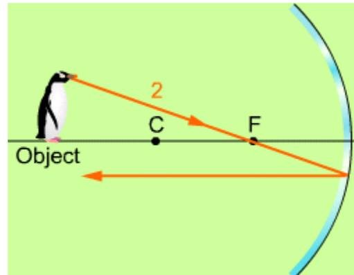
**Ray 2** starts as an incident ray that passes through the focal point and then reflects parallel to the principal axis.
