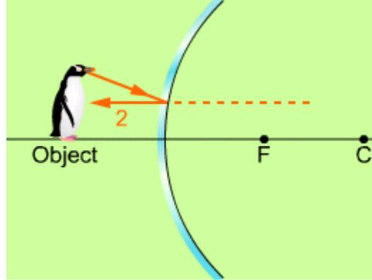
**Ray 2.** Instead of passing through the focal point, the incident part of ray 2 is directed toward it. Before it can reach the focal point behind the mirror, it reflects parallel to the principal axis. Its virtual extension behind the mirror is also parallel to the axis.
