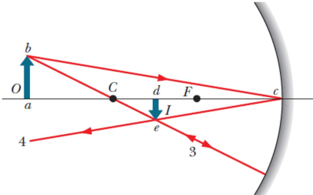
**Ray 3:** A ray that reflects from the mirror after passing through the center of curvature  $C$  returns along itself.
