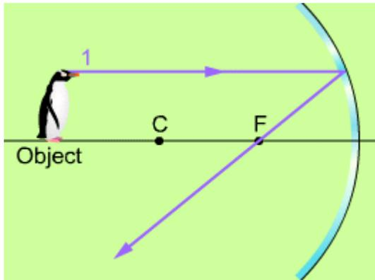
**Ray 1** starts as an incident ray that is parallel to the principal axis. It reflects off the mirror and passes through the focal point after it reflects.
