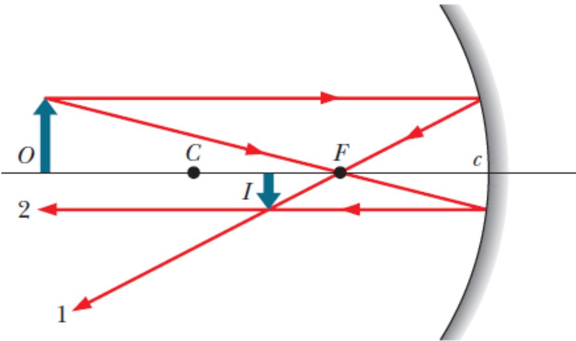
**Ray 1:** A ray that is initially parallel to the central axis reflects through the focal point  $F$ ;
