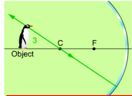
**Ray 3** begins as an incident ray that passes through the center of curvature, strikes the mirror perpendicularly, and reflects back, moving along the same line as the incident ray.
