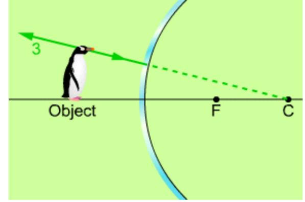
**Ray 3.** The incident component of Ray 3 is directed toward the center of curvature of the mirror and reflects back along the same line. The virtual extension of the reflected ray passes through the center of curvature.
