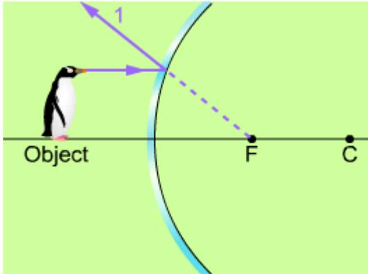
**Ray 1.** Ray 1 is incident parallel to the principal axis. If we extend the reflected component of this ray backward through the mirror, the virtual ray will pass through the focal point.
