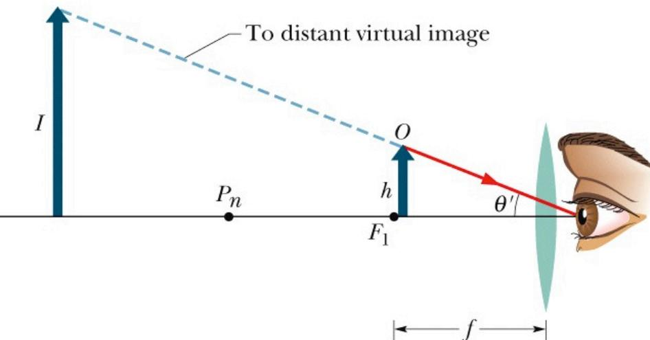
Object at near point  $P_n$ , the angle  $\theta$  corresponds to the ability the eye can distinguish the height of the object.
