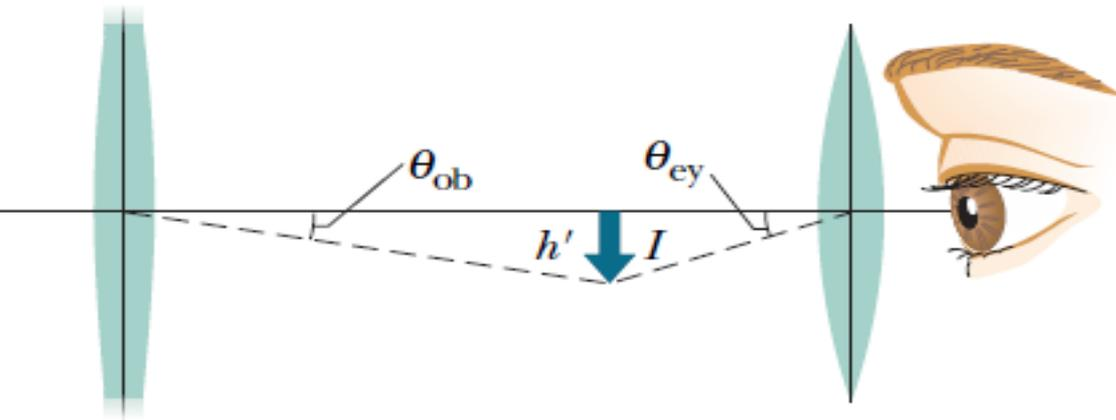
The angular magnification  $m_\theta$  of the telescope is  $\theta_{ey}/\theta_{ob}$ . For rays close to the central axis, we can write  $\theta_{ob} \approx h/f_{ob}$  and  $\theta_{ey} \approx h'/f_{ey}$ , which gives
