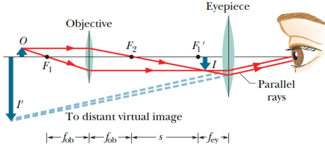
If the lateral magnification produced by the objective is  $m$ , and the total magnification of the microscope is  $M$ , then
