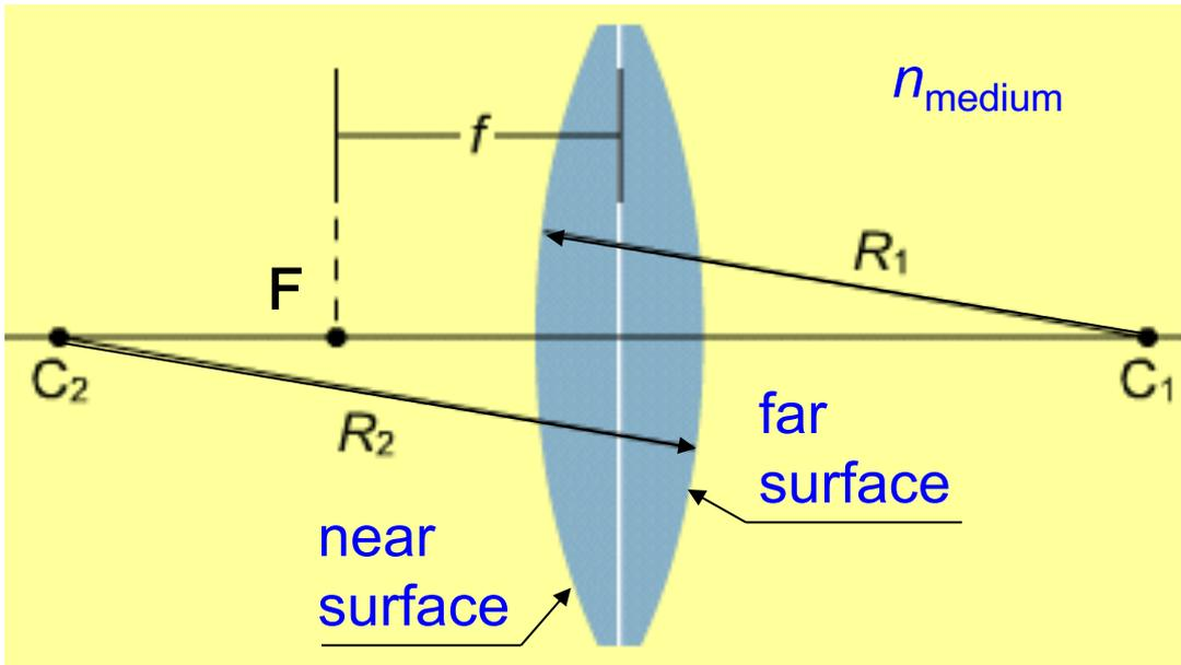
$$\frac{1}{f} = \left( \frac{n_{\text{lens}}}{n_{\text{medium}}} - 1 \right) \left( \frac{1}{R_1} - \frac{1}{R_2} \right)$$
