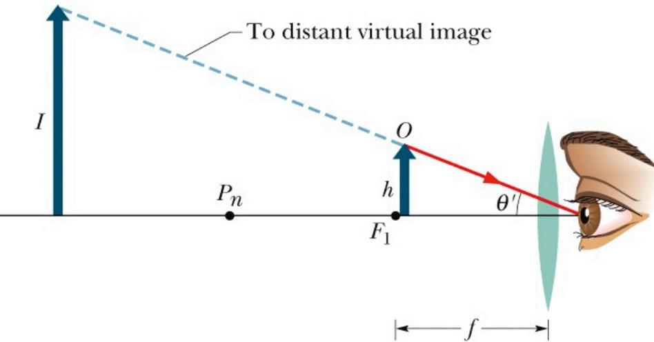
The angular magnification (not the lateral magnification) of a simple magnifying lens is
