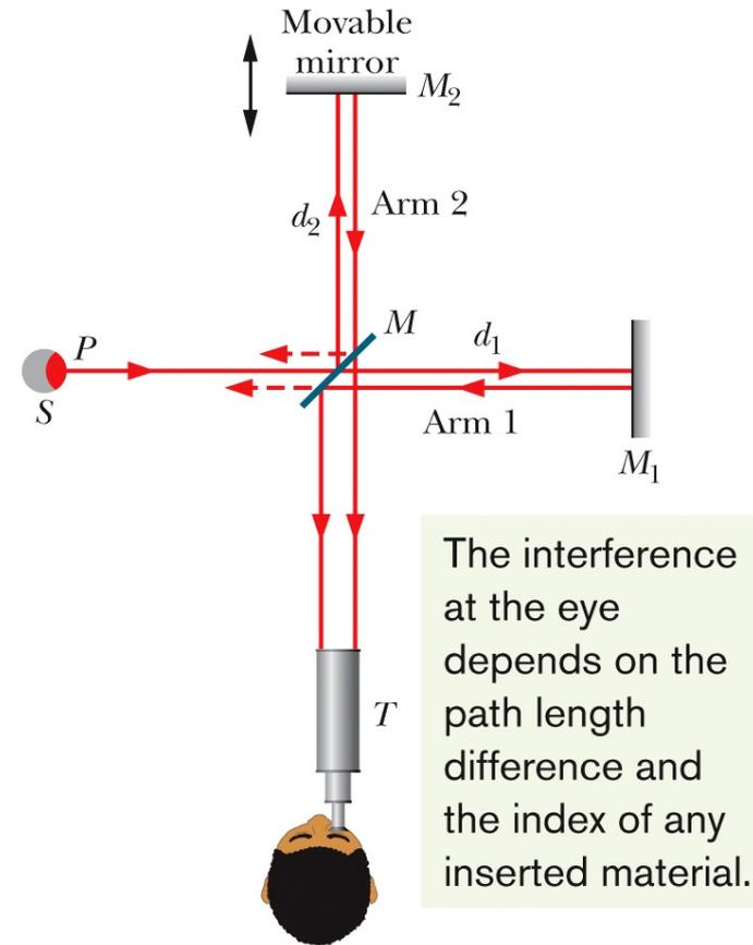
Michelson's interferometer, showing the path of light originating at point  $P$  of an extended source  $S$ . Mirror  $M$  splits the light into two beams, which reflect from mirrors  $M_1$  and  $M_2$  back to  $M$  and then to telescope  $T$ . In the telescope an observer sees a pattern of interference fringes.
